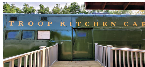
The handicap accessible entrance to the car, through the original service door, is shown above.
