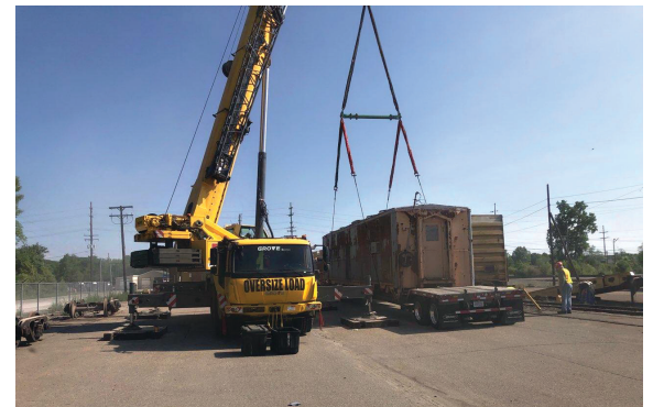
In Flint, the crane lowers the carbody of the Troop Kitchen Car onto the flatbed truck of the semi in preparation for the move to Port Sanilac.
