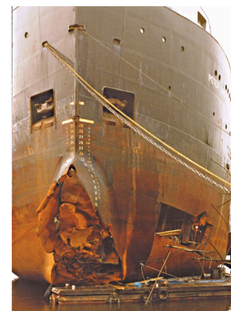
The lower Saguenay River is a fjord carved out by glaciers. The view was spectacular with rock walls towering on either side of the river – and then the Misener collided with the side of the mountain. The Misener is shown here in Montreal awaiting repairs.
