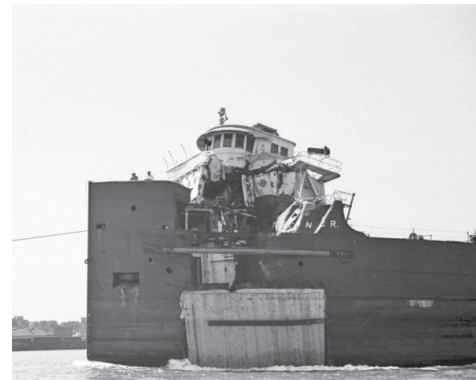
The J. P. Morgan, being towed through the St. Clair River. The temporary patch on the hull can be seen. Courtesy of Wayne “Skip” Kadar’s book, Great Lakes Collisions, Wrecks and Disasters, Ships 400 to 998 Feet, originating from the Russell Sawyer Collection of the Port Huron Museum, Port Huron, Michigan.
